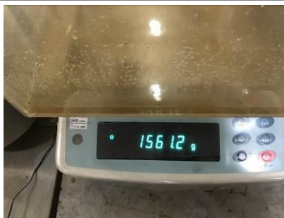
Through-seat leakage (During burn period)
