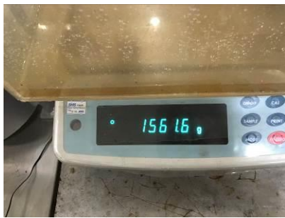
Through-seat leakage (After cool-down)
