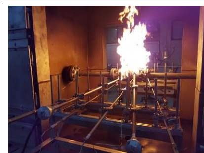
Fire test for DBB Valve - Burning (2" Class 150, API 607)
