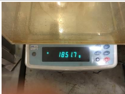
Through-seat leakage (During burn period)
