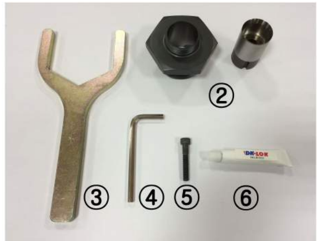
② DJS consisting of DIE and JIG ③ Ratchet Wrench ④ Allen Key ⑤ DIE Fixing Bolt ⑥ DKLUB-0311 (Lubricant)
